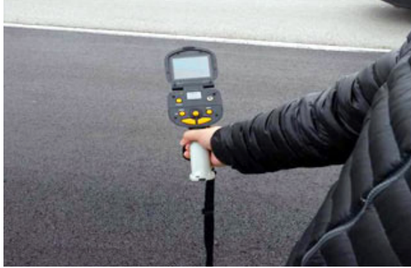
Fig. 5 Asphalt Mat Temperature Measurement Using IR Camera
