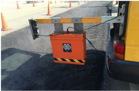
Fig. 3 GPR Test during Construction
