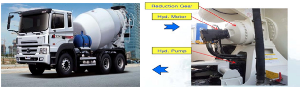
Fig. 1 Drum capacity, 6~8m 3 class concrete mixer truck and driving-related parts of the mixer drum
