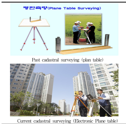
[Fig. 1] Comparing of past cadastral surveying and current cadastral surveying[12]
