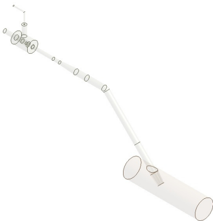
[Fig. 4] 3D modeling of flow region of air-liquid ejector
