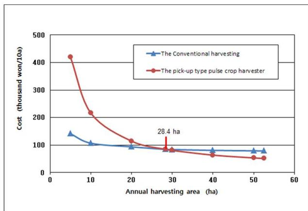
**Figure 2.** Changes in costs per 10 a based on annual harvesting area increases for soybean.
