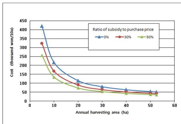
**Figure 5.** Changes in costs per 10 a of the pick-up type pulse crop harvester when a government subsidy is and is not provided to purchase the harvester for soybean harvesting.
