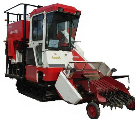
Figure 1. Overview of pick-up type pulse crop harvester.
