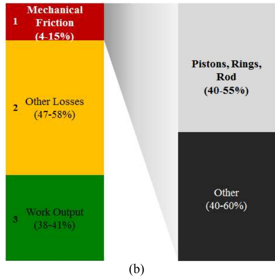
Fig. 1 Schematic diagram of the piston-cylinder and Distribution of total energy and total engine mechanical friction
