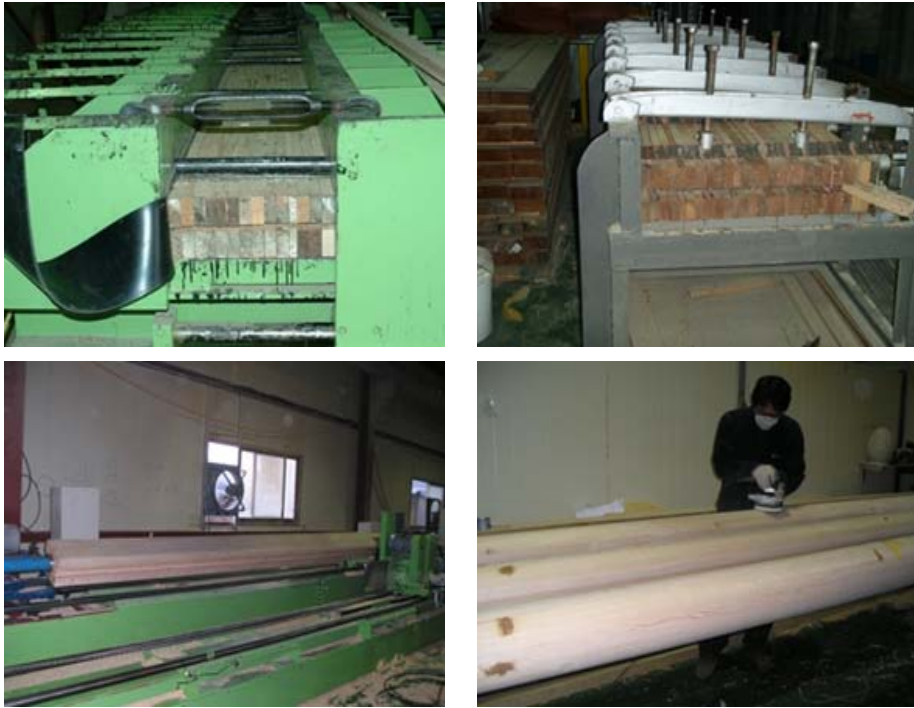
Fig. 1. Manufacturing process of cylinder laminated timber.
