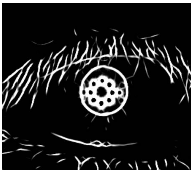
Fig. 23B. Convolution result with twenty gabor filters
