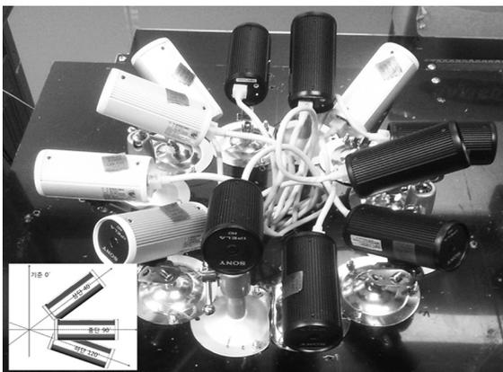
Fig. 3. Alignments of 12 IP cameras
