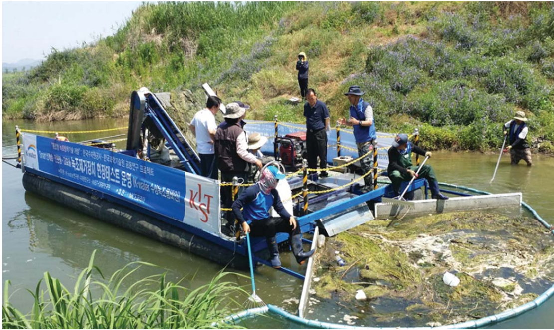
Fig. 3. A photograph showing the elimination of massive algal scum by K-water GATE water combine near the Ugok bridge of the Nakdong River on May 2014.
