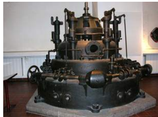
Fig. 2. Holzwarth Experimental Gas Turbine [14]
