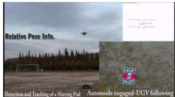
Fig. 8. Flight test result of the moving target tracking
