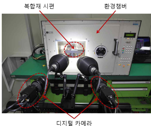
Fig. 2. Arrangement of environment chamber and two digital cameras
