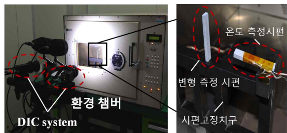
Fig. 8. Specimens for measuring CTE and temperature
