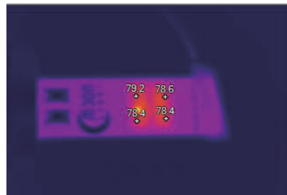
Fig. 10. Temperature contour of a LED headlamp with IR camera.
