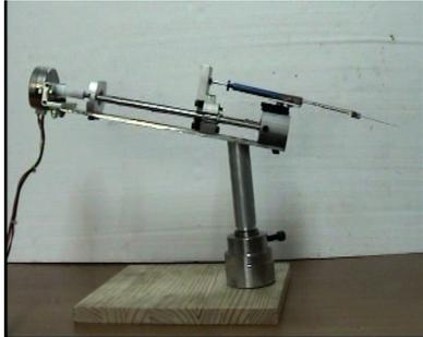
Photo. 2. Step motor, microsyringe and rotational profile.
