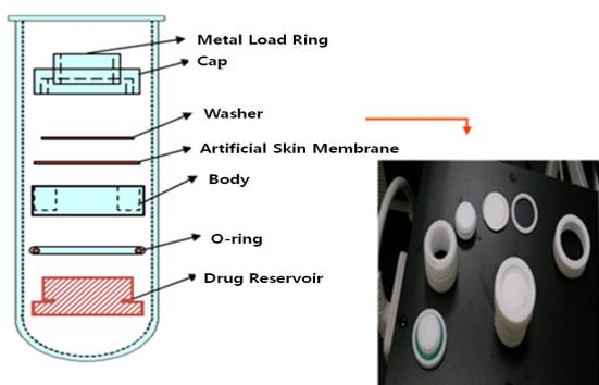
Fig. 7. Thermo-sensitive smart sensor DDS measuring equipment.
