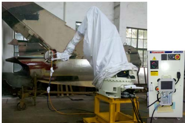
Fig. 7 Six axes robot operating in airplane paint removal site
