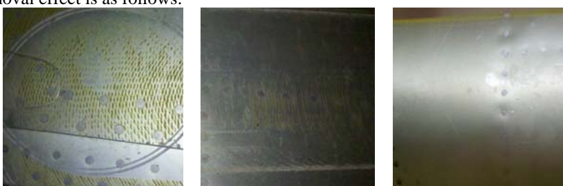
a ) Paint removal effect under 2.4m/min and different pressure
