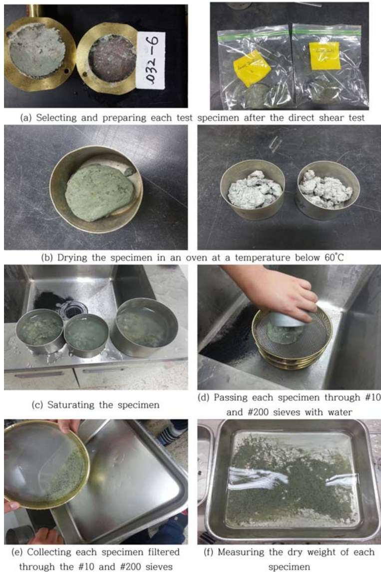
Fig. 5. Sieving procedures to weigh each size fraction after the direct shear test.
