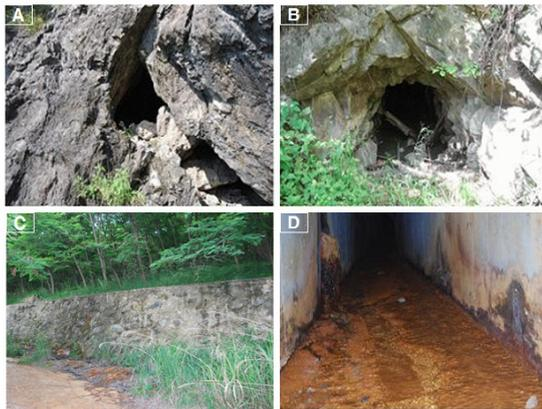
**Fig. 2.** Photographs of main AMD occurrence of Janggun mine area. (A and B) Collapsed and open mine adit. (C) Tailings planted with acacia. (D) Brownish yellow precipitates in waterway.
