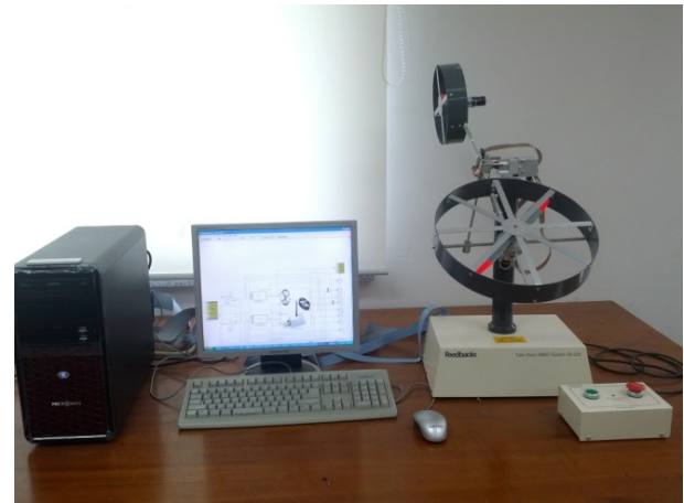
Figure 4. Twin rotor multi-input-multi-output system in laboratory.
