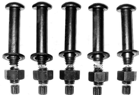
Fig. 11 Specimen after Broken(rust condition)
