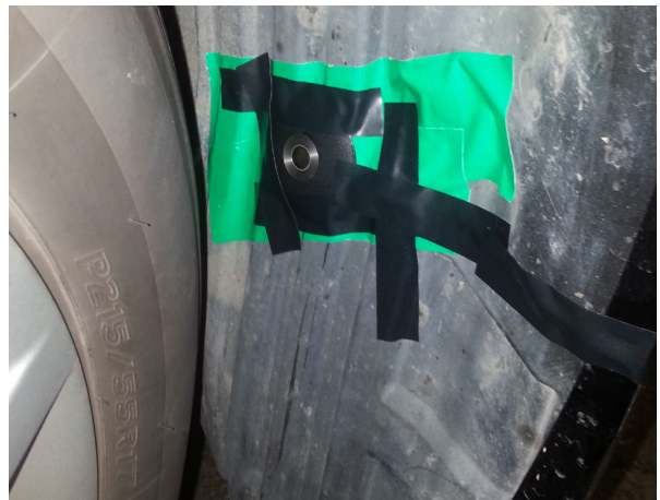
Fig. 1 Installment of a Surface Microphone
