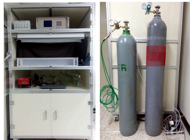
(a) Nox Removal Efficiency Tester (b) Synthetic Air and NO Source (NO 300ppm/N 2 )
