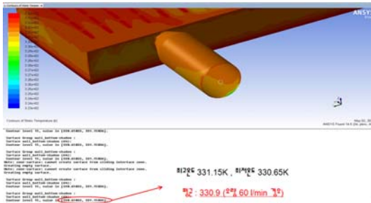
Fig. 7 Outlet Temperature of A Type Cooling System
