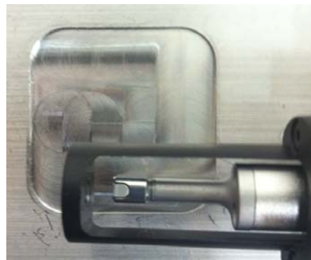
Fig. 3 Surface roughness measurement
