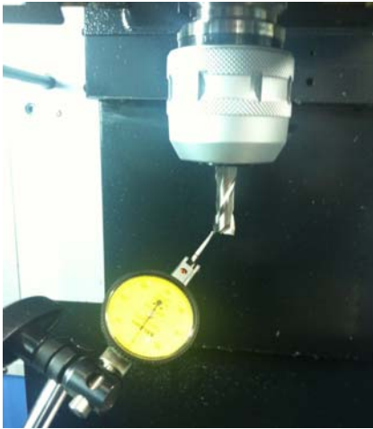
Fig. 1 Runout check for HSS endmill
