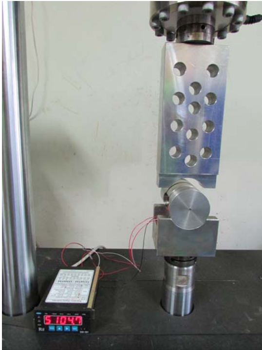
Fig. 13 Using the digital weighing indicator test
