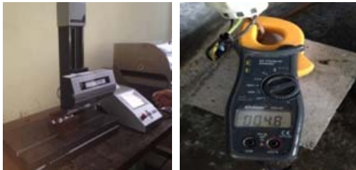
Fig. 3 Measurement equipment (a) surface roughness, (b) AC clamp-On Ammeter
