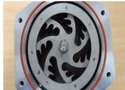
Fig. 1 Shape of turbine blade
