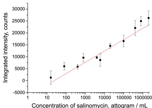
**Figure 3.** Experimental plot of the <sup>49</sup>Ti intensity measured by ICP-MS vs the concentration of salinomycin (3 repeated measurements).
