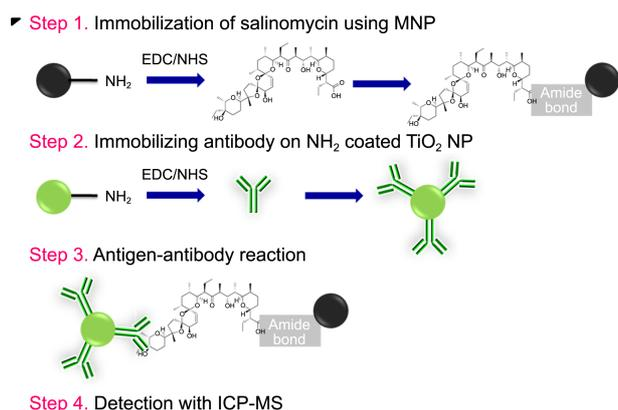
**Figure 1.** Scheme of the experimental procedure for the detection of salinomycin using magnetic and TiO<sub>2</sub> particle tagging.
