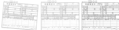
(a) Original (b) Skew-corrected (c) Binarization (Figure 4) Preprocessing Results for Tax form image
