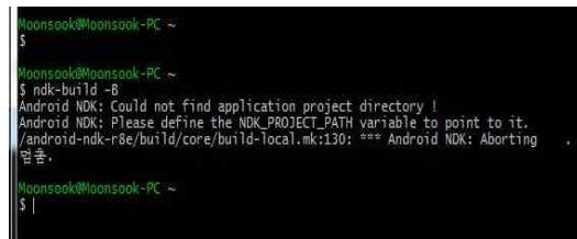
(Figure 3) Result of 'ndk-build -B'
