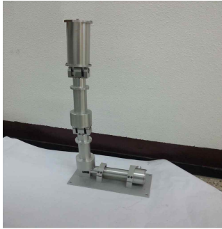
Figure 5: Developed 4-axis waterproof robot arm
