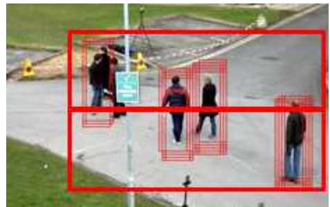
Fig. 6. Parallel processing implementation of pedestrian detection based on ROI-CENTRIST (odd frame)
