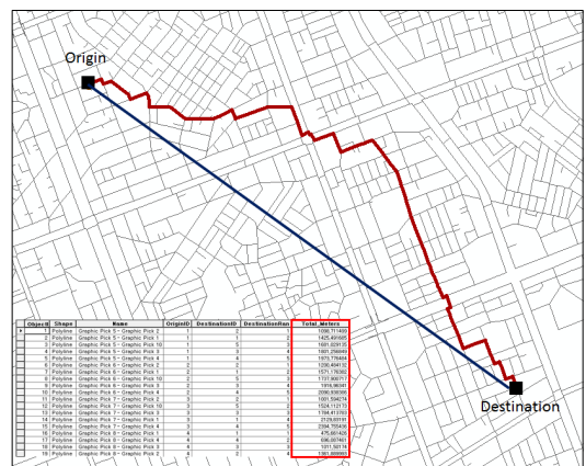
Figure 3. Characteristics of OD Cost Matrix Module (Example)
