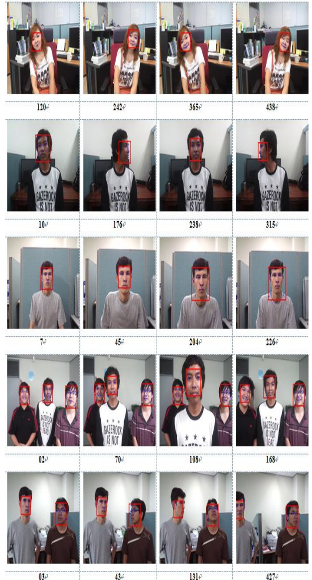
Fig. 6. Results of the proposed face tracker with several different scenarios, 1st row: free moving style, 2nd row: rotation, 3rd row: scaling, 4th row: multi-face scaling, 5th row: multi-face rotation
