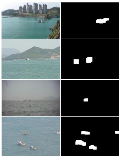
Fig. 4. Result of morphological "close" operation and thresholding.
