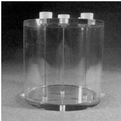
Fig. 3. Triple line phantom was used to evaluate the resolution of SPECT.
