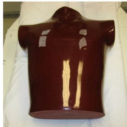
Fig. 4. Anthropomorphic chest phantom was used to evaluate noise and exposure dose of CT.
