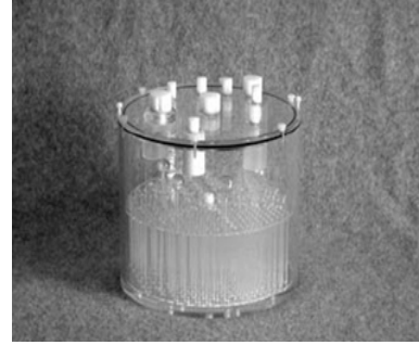
Fig. 2. Flangeless Esser PET phantom was used to evaluate of % contrast of SPECT.
