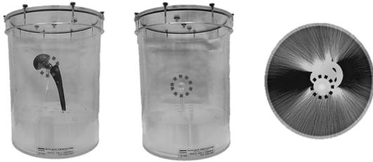
Fig. 1. Artificial hip joint was inserted to SPECT/PET phantom, 17 mm sphere of Bright Streak area in CT image was filled with Tc-99m so that the radiation activity was 8 times compared to background.
