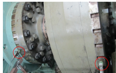
Fig. 4 Gap sensor positions for torsional vibration measurement
