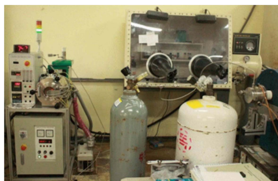
Fig. 1. High frequency Induction Furnace used for synthesizing experiment.
