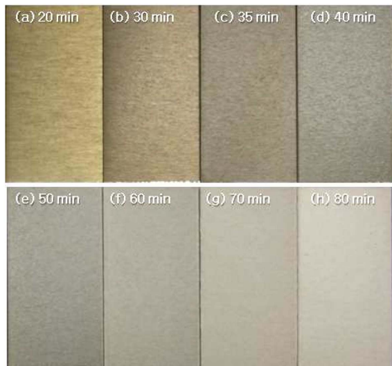
Fig. 3. Photographs of anodized Al7075 alloys with anodization time at 40 mA/cm 2 in 20% H 2 SO 4 solution.
