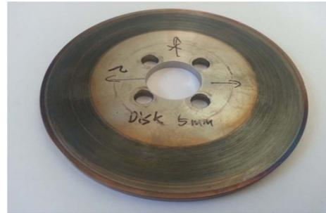
Fig. 8. Morphology of disk surface after test for 5 mm disk.
