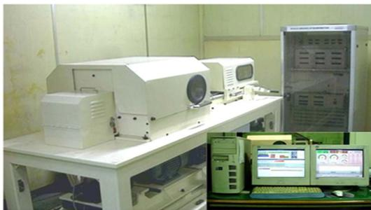
Fig. 3. Lab-scale dynamo tester.
