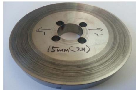
Fig. 10. Morphology of disk surface after test for 15 mm disk.
