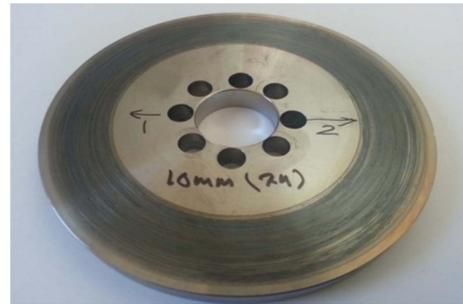
Fig. 9. Morphology of disk surface after test for 10 mm disk.
