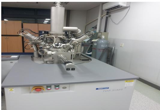
Fig. 1 SIMS apparatus for measuring a black Cr solar selective coating
