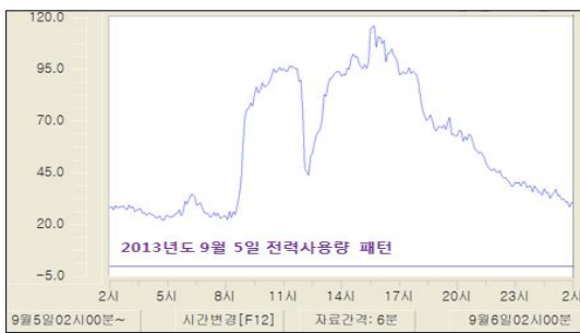
(b) 2013.9.5. Building power consumption pattern
