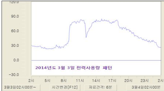
(c) 2014.3.3. Building power consumption pattern
