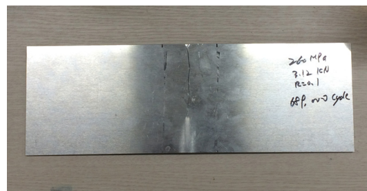
Fig. 2 The plate specimen through 3 point bending fatigue test
