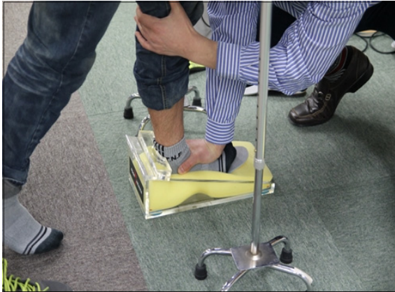
Fig. 2. Experimental Insole production process
