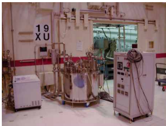
Fig. 2. LN2 circulation cooling system (cryocooler-cooled type) for spectrometer. Circulating LN2 temperature: 66 K - 81 K, Cooling power: 0.3 kW - 1 kW, Flow: 5 L - 15 L/min, \Delta P : 70 kPa.
