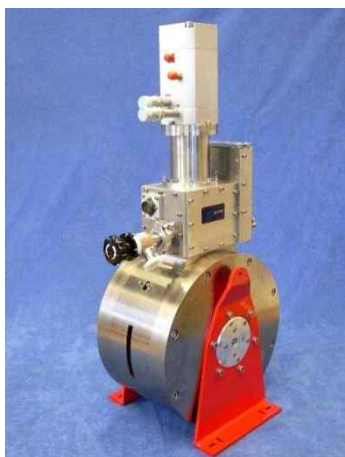
Fig. 6.1. HTS dipole magnet. Taking advantage of the HTS, this high-speed ramping magnet performs a cycle (0, 7 T, -7 T, 0) in less than 320 s. Used in Kerr effect measurement devices.
