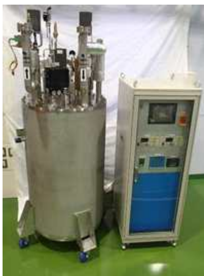
Fig. 1. LN2 circulation cooling system (bath-cooled type) for spectrometer. Circulating LN2 temperature: 78 K, Cooling power: 2 kW, Flow: 5 L - 20 L/min, \Delta P : 0.3 MPa.
