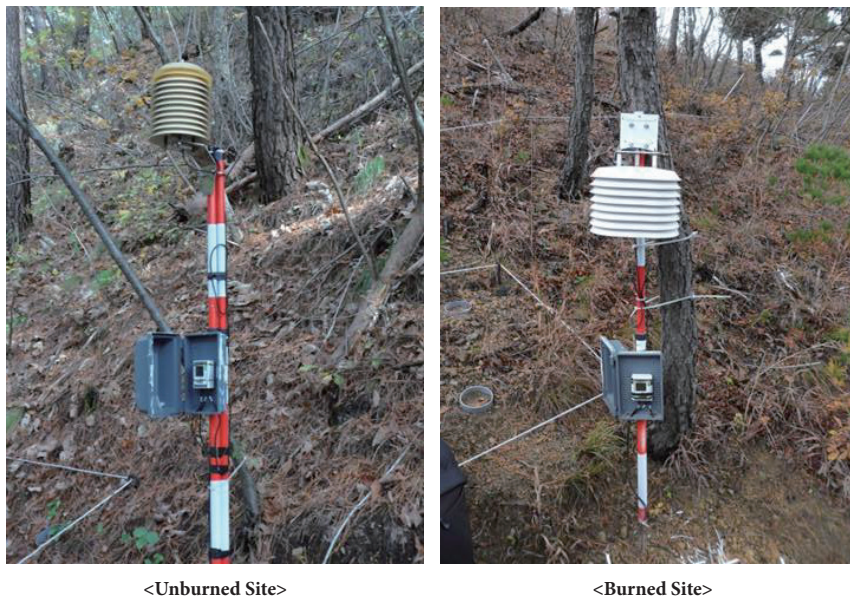
Fig. 4. The installation photographs of data logger used in this study.
