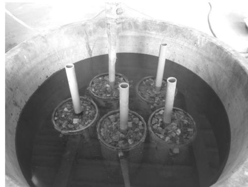
Fig. 6. Preparation process of specimens for compressive strength test
