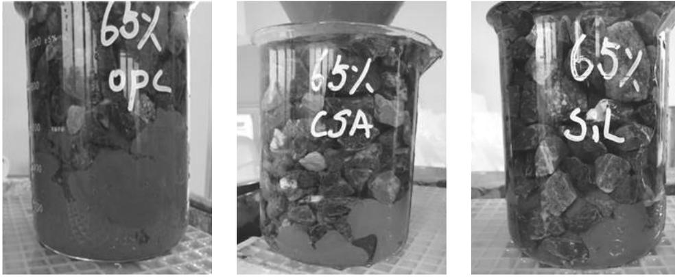
Fig. 3. Quality confirmation of grout materials by visual inspection
