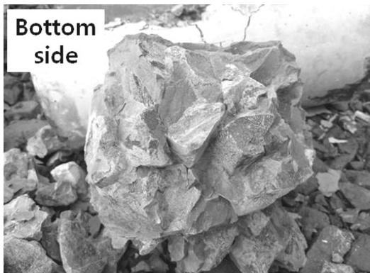
Fig. 5. Segregation of aggregate after curing (Portland cement with 0% of anti-washout admixture content)
