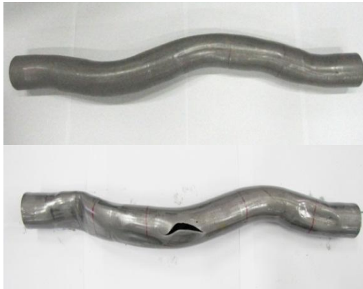
Fig.12 Defects at trailing arm shape
