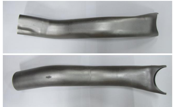
Fig.14 Hydroformed trailing arm after end cutting
